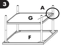
**STEP THREE:** Once the **cart legs** (**E**) are fully installed, fasten the **LOWER SHELF** (**G**) to the second half of the **cart legs** (**E**) using the longer **screws/washers** (**A**).
