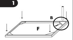
STEP ONE: Grab the UPPER SHELF (F) and flip it upside down. Install the one half of the cart legs (E) that have one hole. Fasten legs to UPPER SHELF using the provided allen key (C) and the shorter set of screws/washers (B).
