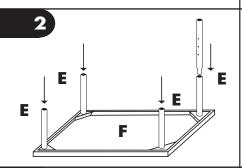
**STEP TWO:** Install the second half of the **cart legs (E)** into the first half.
