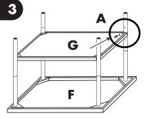
**STEP THREE:** Once the **cart legs** (**E**) are fully installed, fasten the **LOWER SHELF** (**G**) to the second half of the **cart legs** (**E**) using the longer **screws/washers** (**A**).
