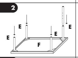
**STEP TWO:** Install the second half of the **cart legs (E)** into the first half.
