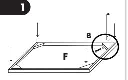
STEP ONE: Grab the UPPER SHELF (F) and flip it upside down. Install the one half of the cart legs (E) that have one hole. Fasten legs to UPPER SHELF using the provided allen key (C) and the shorter set of screws/washers (B).
